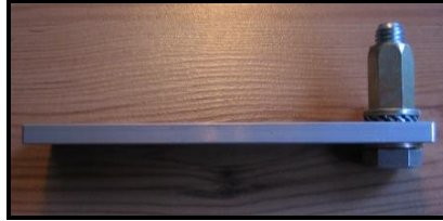
Picture A: Rivet nut install tool fully assembled and ready to go.
