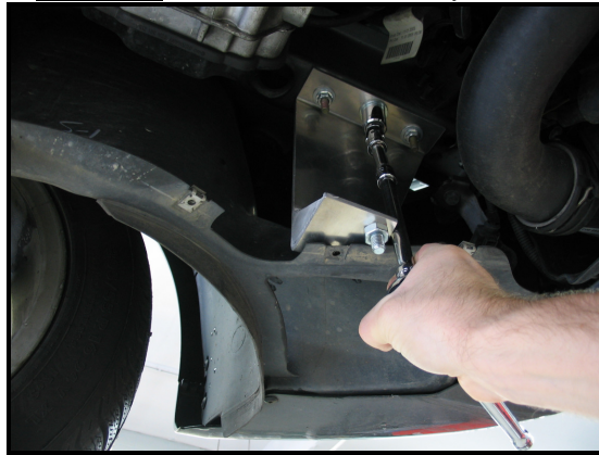
Picture E: Drivers side bracket fully installed.
