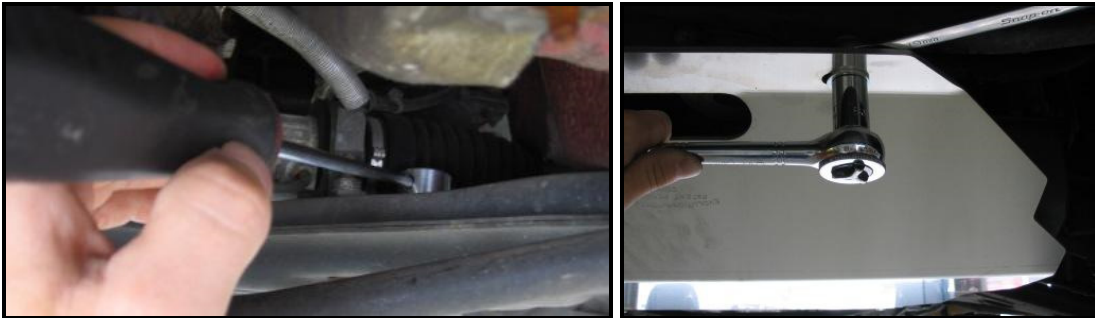
Picture D: Tightening the rear mount.(Left) Tightening the front mount.(Right)
