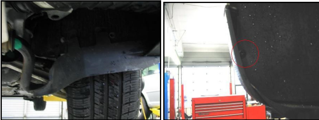
Picture B: Plastic lip that needs to be removed (Left) and Torx screw in the fender liner (Right).
