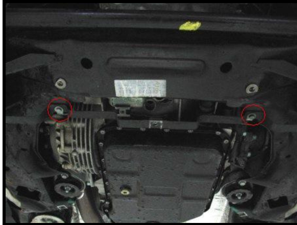
Picture A: Metal bracket that needs to be removed.
