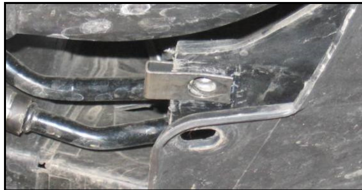
Picture G: 8mm speed clip installed.
