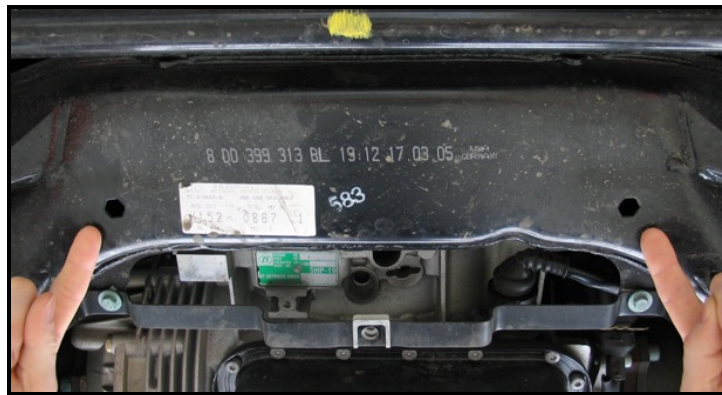
Picture B: Location of where the two Rivet-nuts will be installed on the rear sub frame.
