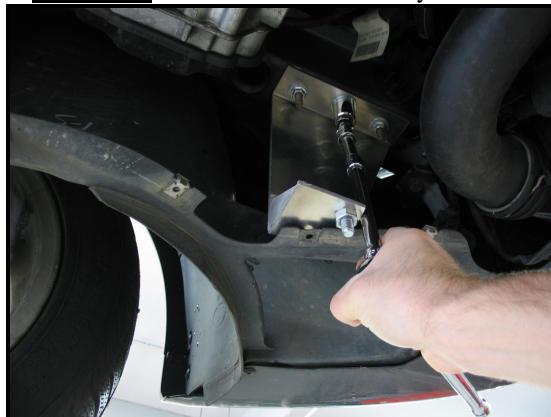
Picture G: Drivers side bracket fully installed.
