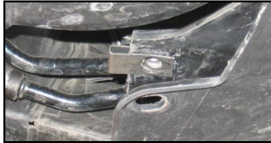
Picture G: 8mm speed clip fully installed.
