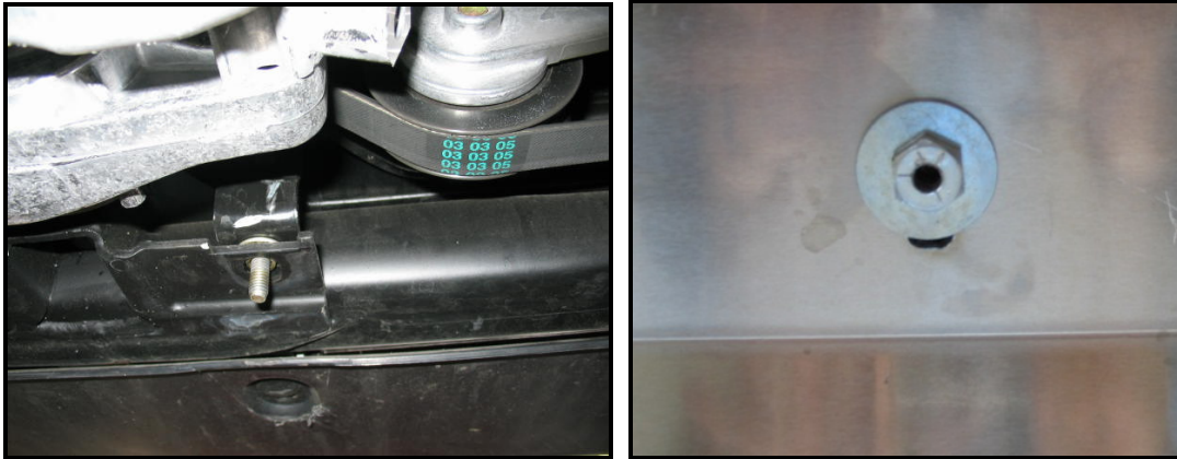
Picture I: Stationary bolt. (Left) 6mm internally threaded bolt installed. (Right)
