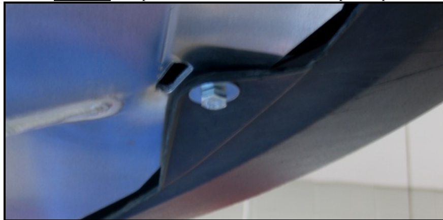
Picture J: Skid plate bolted to one of the two front speed clips.
